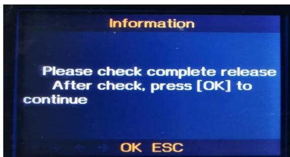
11. The entire process is completed. Depress brake pedal and hold depressed. Activate the electromechanical parking brake button -E538 once, release in direction (press button). And then activate the electromechanical parking brake button -E538 once, release in direction (press button). Finally, enter 0053-Parking Brake or 0003-Brake 1 system, read and erase fault codes. And ensure there are no fault codes in control module.
