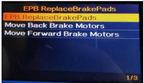
4. Select EPB ReplaceBrakePads, click on the menu, To perform the brake pad replacement function, press OK. To exit, press ESC.
