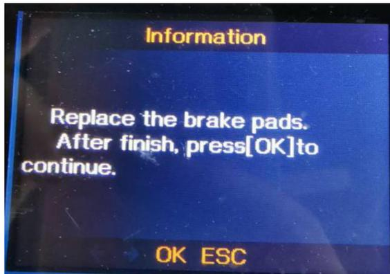
8. The function of Move Forward Brake Motors has been performed and press [OK] button to continue.
