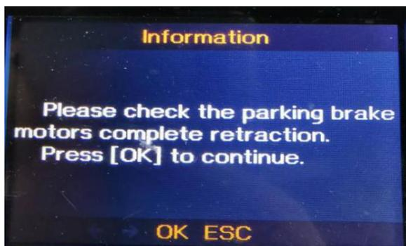
7. Now begin to replace the brake pads. After finish,press [OK] button to continue.
