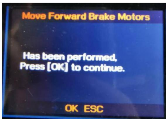
10. Check the brake motors complete move forward and press [OK] button to continue
