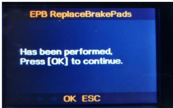
9. Check the brake motors complete move back and press [OK] button to continue
