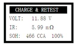
The result indicates the battery is OK and remains 73% of life. But only 11.88V left and over low voltage, which can affect the result. At this time it is better to charge prior to checking again.
