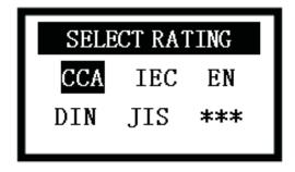
(4) According to the value indicated on the battery, press < > < > button to adjust the reference value of the battery. Long press < > < button to adjust the number continuously. See the picture:
