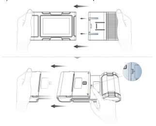
Hold the printer in your hand, aim at the lead-in slot on the back of the main unit, push it in slightly, and you will hear a
