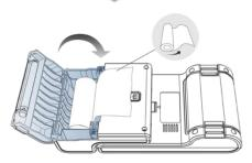
Hold the position of the printer paper bin cover with your fingers and open the cover up;
