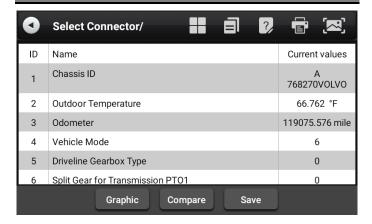
Graphic: View the real-time operating parameters of the unit in the data stream waveform graph mode, and select [List] to return to the numerical display state.
